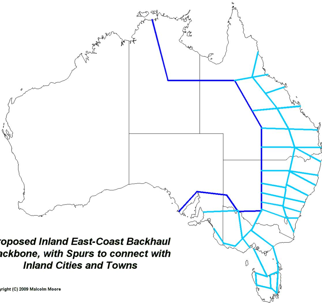
In this case, the Royal Blue line represents a Proposed major Backhaul Backbone, and the Cyan (Light Blue) lines represent Backbones that connect between major centres. This structure forms a grid, so that a number of highly reliable network Rings can be intersected, so that traffic can be automatically bypassed if any of the Backbone routes or Spurs suffer damage.
