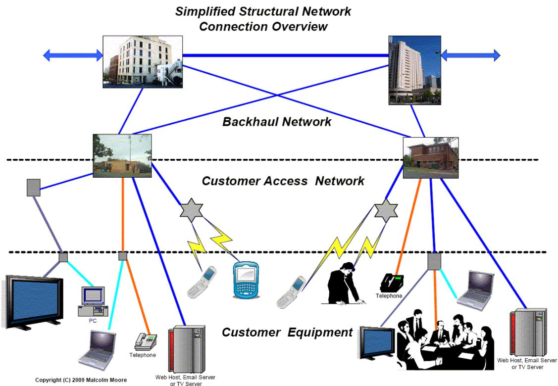
In cases where the distant end is an IP Phone, the VoIP will pass through the Backhaul Network/IPN to the distant Backhaul Network/IPN-CAN router/switch
