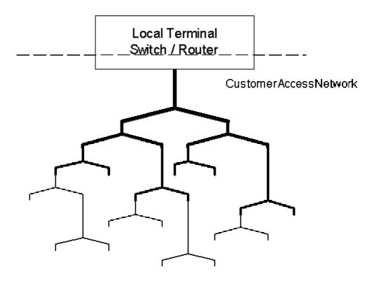
The figure above gives a visual of how cables that leave a Local Terminal site start off quite fat (for example 800 pairs in one cable), and are joined with smaller cables and finally 2-pair (quad) feeding off to households.
