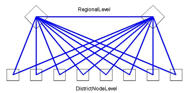
The general structure of networks at the Regional level look like this (above) where each District Node is connected directly with the Regional Switch/Router, and the Regional Switch/Routers are connected (usually in pairs) at the regional level for alternate path routing. In metropolitan areas these paths are usually physical optical fibre (because the lengths rarely exceed 30 km) and these are capable of at least 1Gb/s (if not 10 Gb/s)
