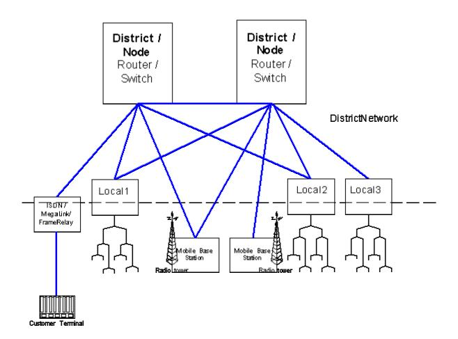
This is a diagrammatic visualisation of a District network connecting with ISDN / MegaLink / Frame Relay / Customer Wideband services, Local Terminal exchanges and Mobile Base Stations. It is only representative, but it shows links to various CAN interfaces connecting through into the District network.
