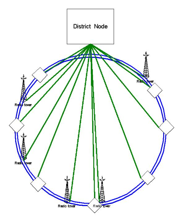
This diagram tries to explain the paradoxical structure where the Blue Rings represent the physical SDH system on a pair of Optical Fibres forming a ring, (with Network Elements along the path); but the configuration of the SDH system in this case is a simple star with every network element being terminated at the District Node site.
