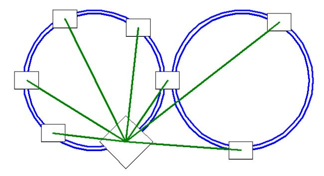
This picture shows two transmission rings that intersect at a District Node site and all the virtual paths are connected to the Regional Switch/Router site. This could well be part of a much larger structure where there are other virtual paths to an alternate Regional Switch/Router.
