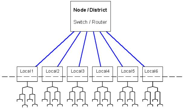
This is a visual of a simple District Network where there is one District Node Switch / Router that connects through a number of transmission systems (shown as a thick blue line) to a number of Local / Terminal Switches / Routers. Below the dotted line is the CAN - shown figuratively as a cable splitting off to thinner cables as it nears customer premises. Most non-metropolitan District networks are similar in structure as this (with only one District Node).
