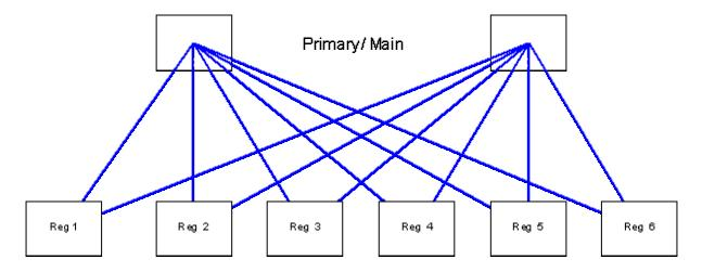
This is the first part of the National Network showing a full inter-level mesh between the Primary / Main Routers / Switches and the Regional Router / Switches. There is also a 'peer level' of connection paths that also exist
