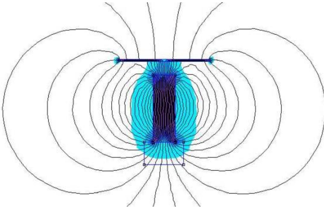
The above picture is a **Finite Element Modelling (FEM)** representation of one of the pickups in the guitar above and the magnetic lines of force and field strength given in a two dimensional picture ('y' – along the string axis (left to right), 'z' vertically through the pickup (bottom to top) of a magnetic guitar string in the vicinity of a small bar magnet.
