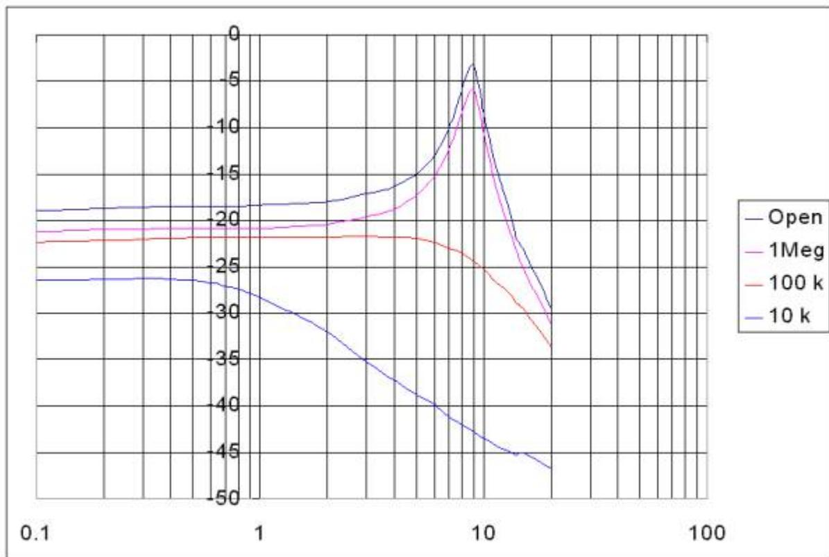
The above graph is the practical results obtained using the Strat 02 pickup with different resistive loads. Referring back to the earlier analysis where predicted values gave almost identical results, it is now clear that all these pickups will follow the same general family of frequency responses, and that response can be predictably tuned by changing the load resistor (and the load capacitor).
