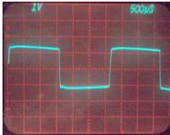
The is the same Strat 01 pickup in the same setup as before but the load resistor is now 10 k ohms. The leading signal edge is considerably smoothed and this is why this has a muffled sound.
