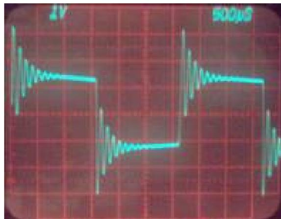
The is the same Strat 01 pickup in the same setup as before but the load resistor is now 100 k ohms. This is a classical step and recovery, void of overshoot.
