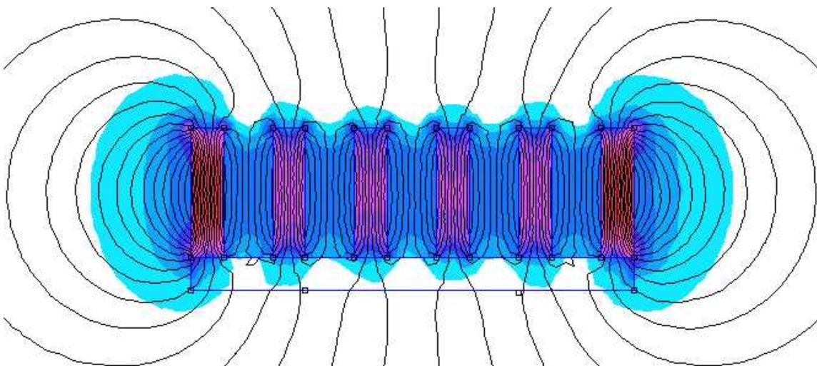
The two pictures above are rather interesting as they show the relative sensitivity of a range of pickups along the face of the pickups, where the strings are numbered 1
