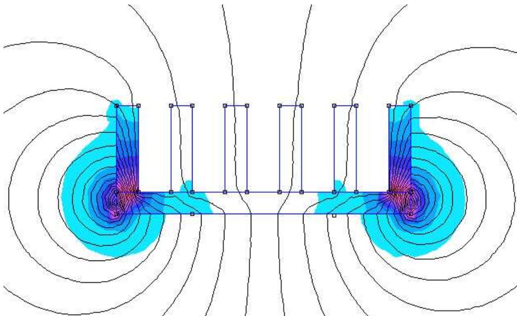
In this case the (ferrite) magnet is sitting under the six soft iron pole pieces and the strings sit a few mm over the soft iron pole pieces. The 2 Dimensional FEM analysis picture above really needs some explanation to tell what is going on:
