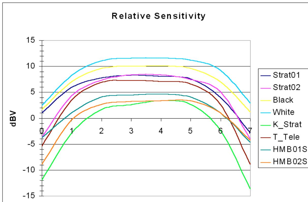
The above graph shows the relative sensitivities of all these test pickups in relation to each other and the overall difference in sensitivity is in the order of 9 dB, which is quite large. I was expecting about 6 dB overall.
