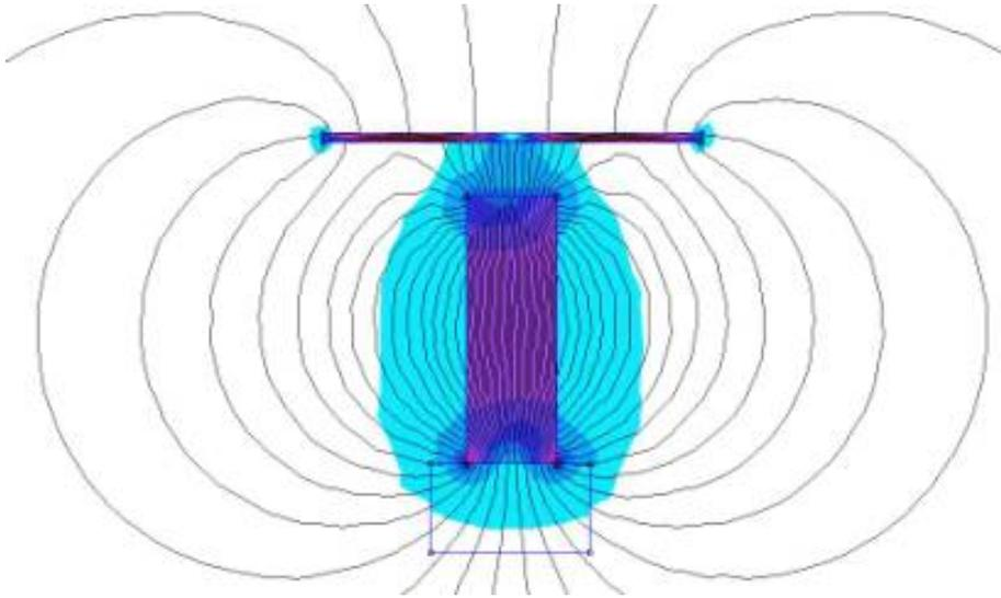
If the North is the top-side and the South is the bottom-side (and it is easier seen if expanded by clicking on it)! On the left hand and right hand ends, the magnetic field is more intense as it wraps itself around the ends to make a circuit – this is happening all along the sides too – but this depiction does not show that - but this is shown in the right hand picture!
