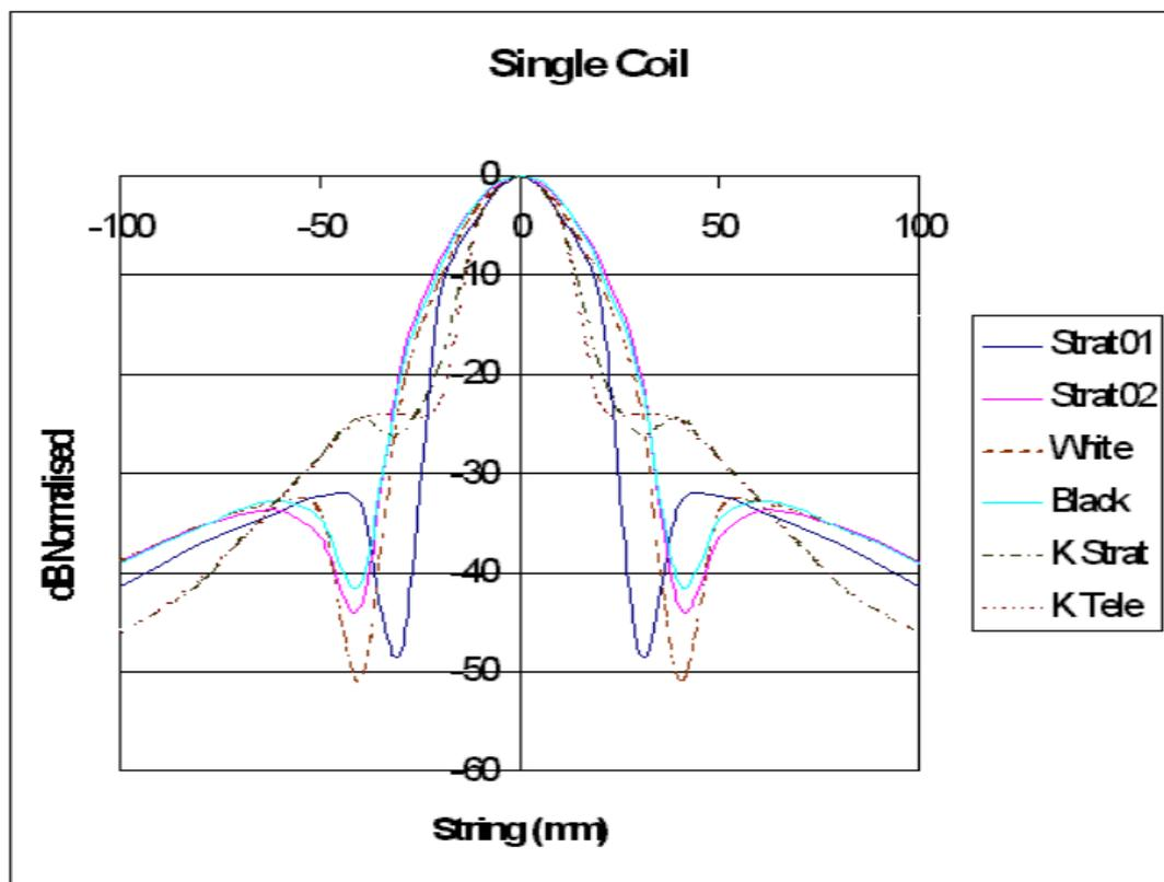
The two pictures above shows the cross-section of the Stratocaster or other single coil pickup and the general sensitivity chart aligned centre of the magnetic field. This should show just how sensitive the relative string movement is, along the string.
