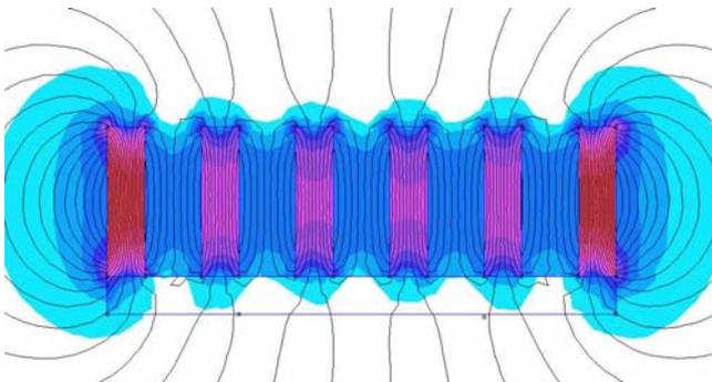
These pictures form an interesting scenario as the six magnets as shown with the 2D map in the lower picture above, have a lot of fields lost between them in magnetic leakage. This 2D picture also indicates that even if the pickup were inverted then the sensitivity could be very similar to the top side.
