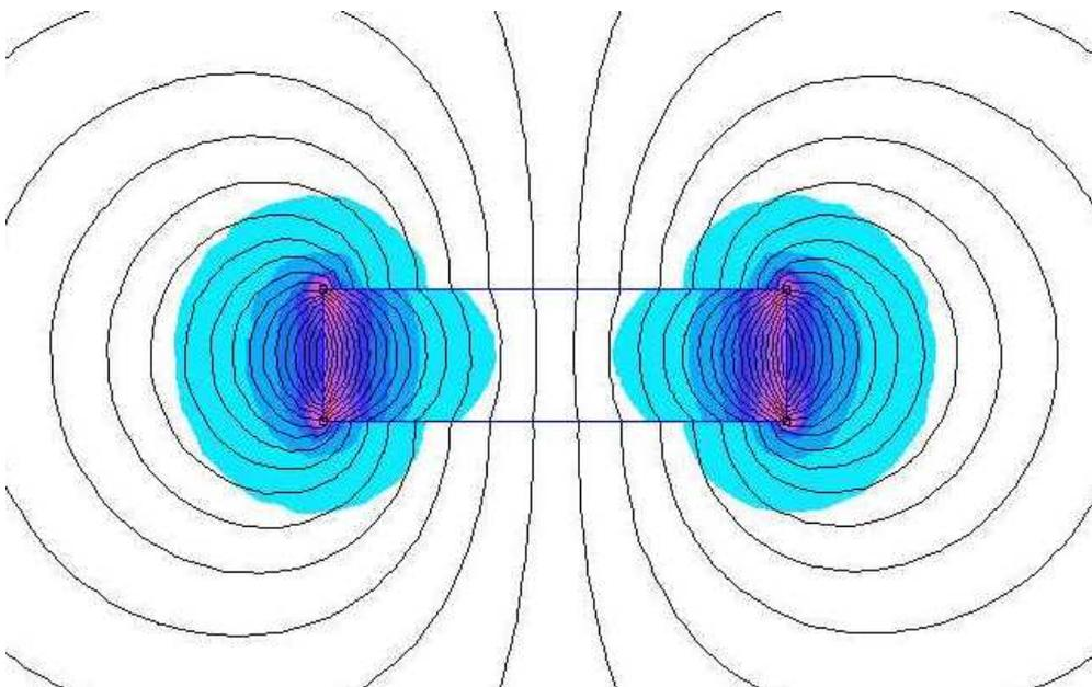
In this case the poles are along the top and bottom of the strip ferrite magnet, and the magnetic field is that seen through the centre of the strip magnet.
