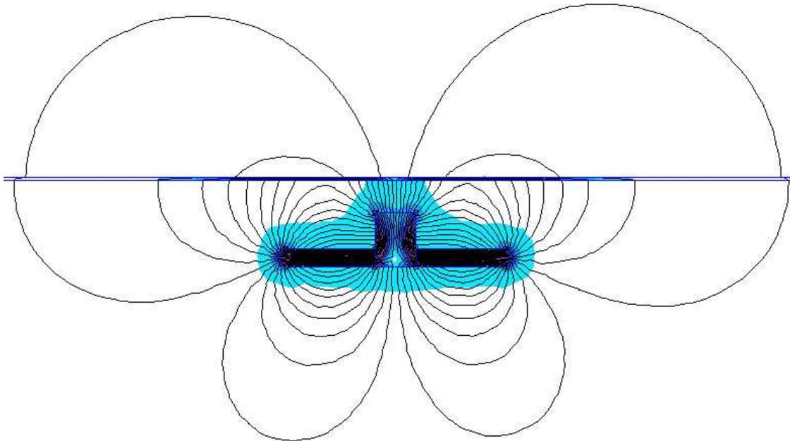
This picture over-justifies the performance capability of the P90 as the centre mild steel square rod is not much thicker than the flat magnets, so the field does not really have that much "carry" into the strings. This analysis does, however open up a large range of innovative ideas for restructuring pickups to be both efficient and sensitive.
