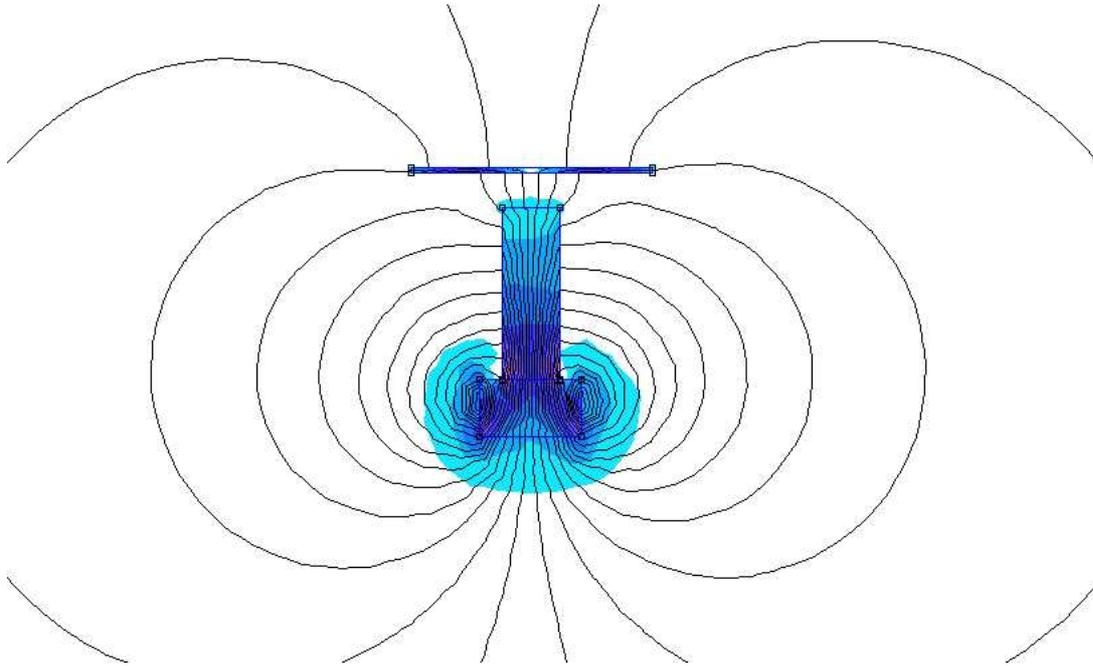
You can see here that there is an intense magnetic field around the edges of the flat bar magnet, and that the north pole (in this case) is extended up through the soft iron rod towards the string.
