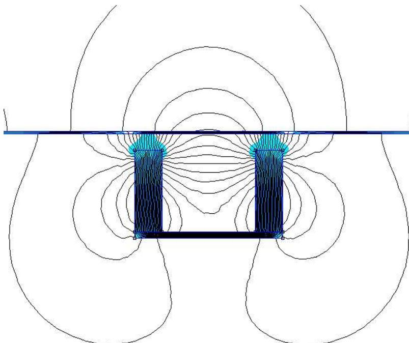
As shown here the vast majority of the stray field is captured and linked to the adjacent rod magnets leaving very little external fields other than that near the strings.
