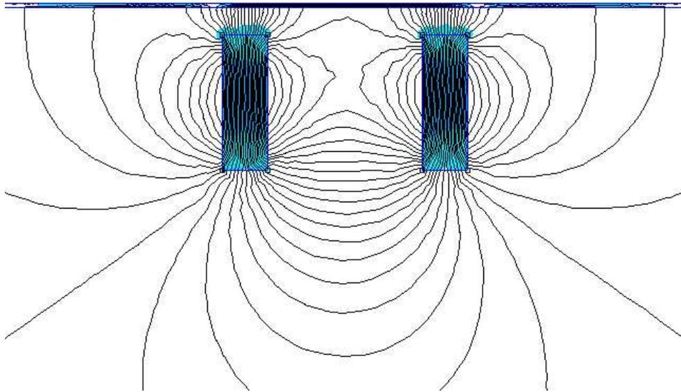
This is not much different that a pair of single magnet pickups put beside one another. The magnetic fields are interacting and pulling into each other to dramatically reduce the amount of external interference. Once a thin iron sheet is placed to join these fields then the large majority of the magnetic fields would pass through the soft iron to again dramatically reduce the external magnetic field.
