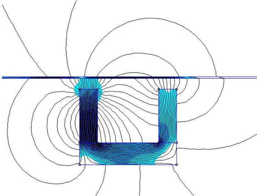
The magnet retains much the same flux density, but the flux density in the now thicker plate is not saturated and the rods on the right hand side are now with a higher flux density, so this simple improvement should make a very significant improvement in the sensitivity of this type of pickup, and its ability to not be affected nearly as much by distant electromagnetic fields.
