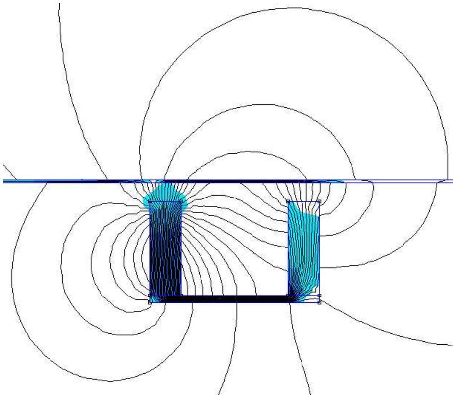
In this case the six bar magnets are mounted on the left hand side and a thin soft iron mounting plate is the lower reluctance path to the right hand side where six soft iron rods form the return path towards the strings through the air.
