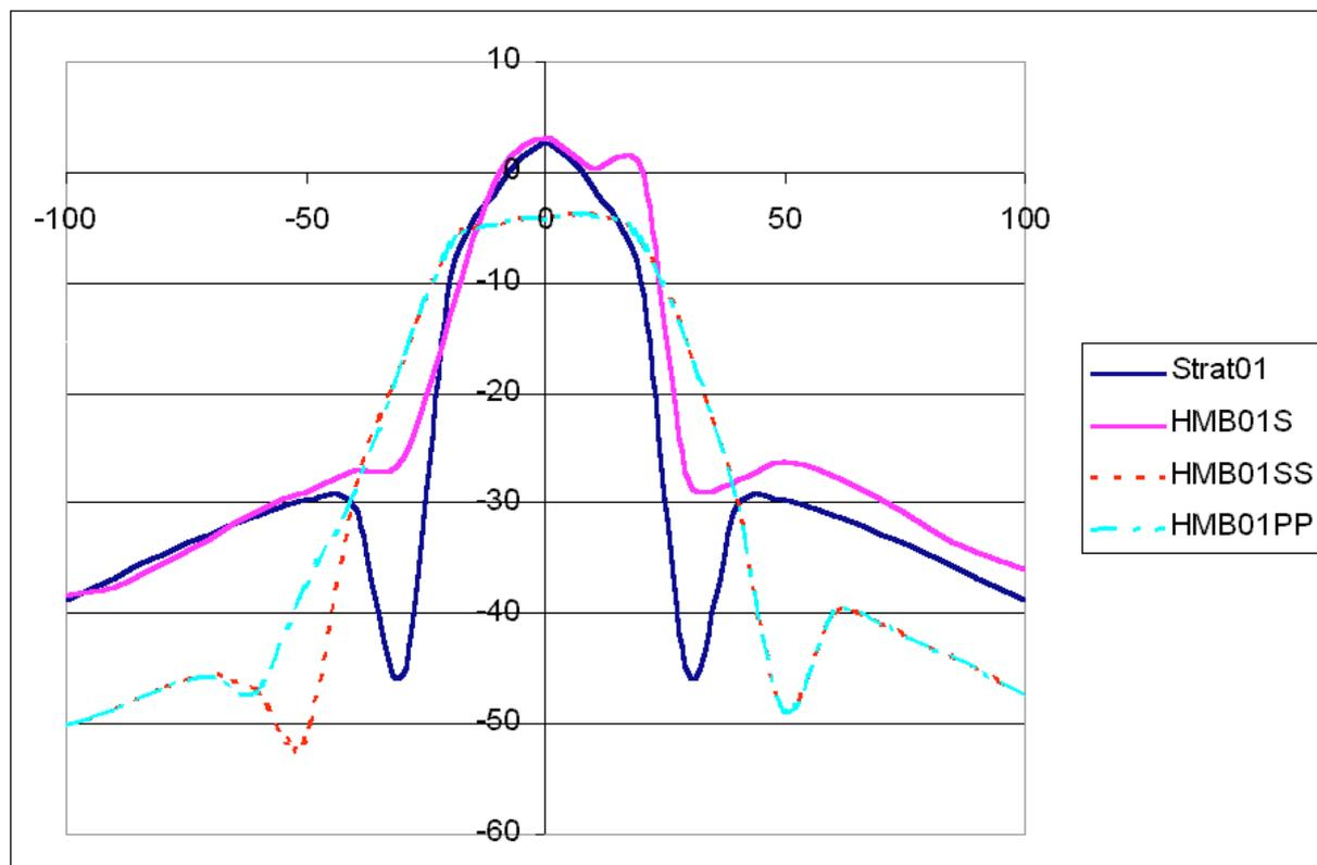
This is particularly interesting as the Strat, and the hum bucker wired as a single (HMB01S) form a nice pair with the extra metalwork of the hum bucker putting a 'bump' on one side of the sensitive curve (caused by the second pole piece).
