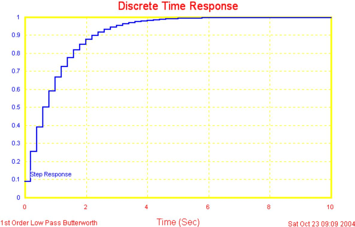
The above time response is a 1<sup>st</sup> order digital response of a 1 Hz Low Pass Filter (Exponential Moving Average) being clocked at 5 Hz. Note the big steps that are coincidental with each sample.
