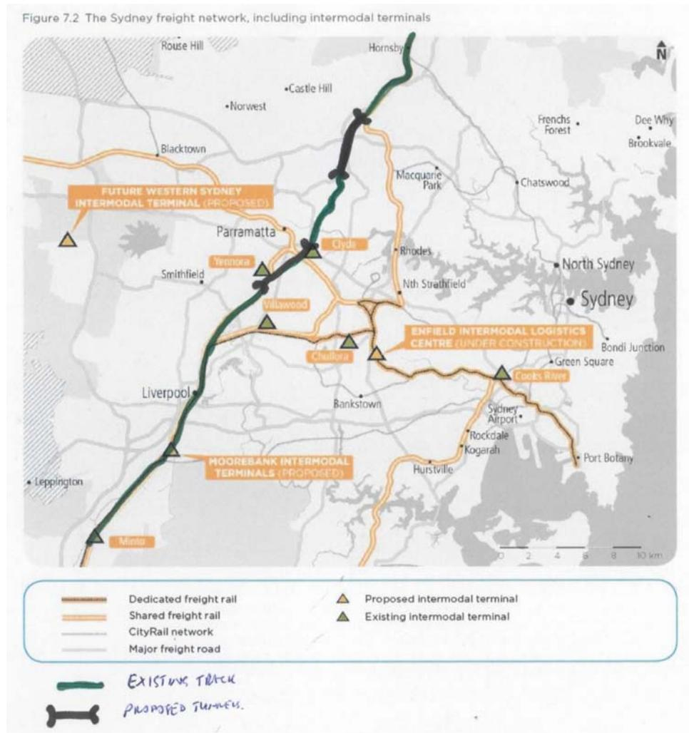
A relatively quick investigation of this situation showed me that it would be rather easy to position two nominally 4 km tunnels and join some rather underutilised existing rail infrastructure to directly connect Liverpool to Hornsby such that a quick rail freight train could traverse this nominal 37 km span in about 22 minutes. A short document<sup>9</sup> on this subject was recently forwarded to the Master Plan Team
