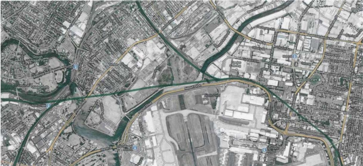
The picture above shows the proposed rail alignment corridor path as a thick green line over the south of Mascot and from a branch line pair just north of the Airport, over the Princes Highway towards Wollie Creek station into the East Hills line.
